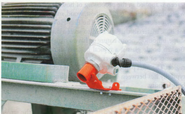
4 Sensors can be used to back the blade away during stoppages or when running empty
