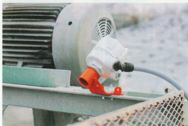
4 Sensors can be used to back the blade away during stoppages or when running empty
