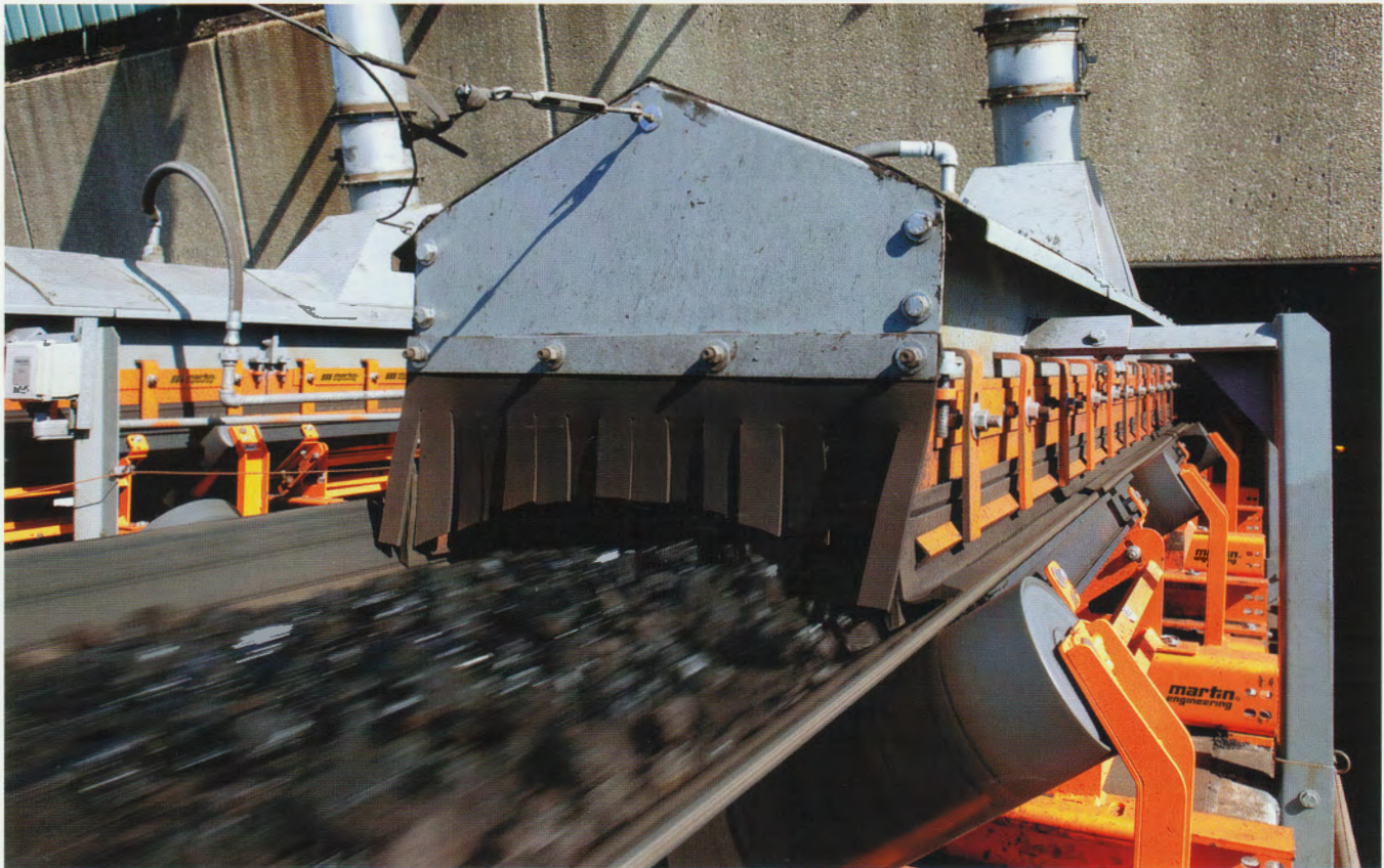
7 Transfer point with enclosure, support, skirt sealing and dust curtains
