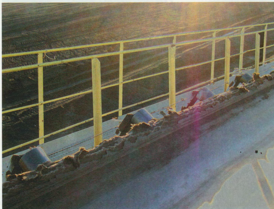
6 Belt edge damage from mistracking
