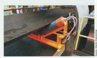
3 For locations without electricity or plant air, the Roll Generator creates its own mini-power station
