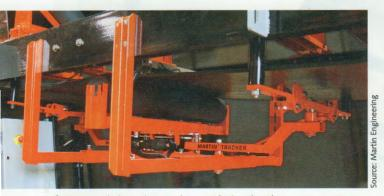
1 The new belt tracker can be specified with either a pneumatic or electric actuator
