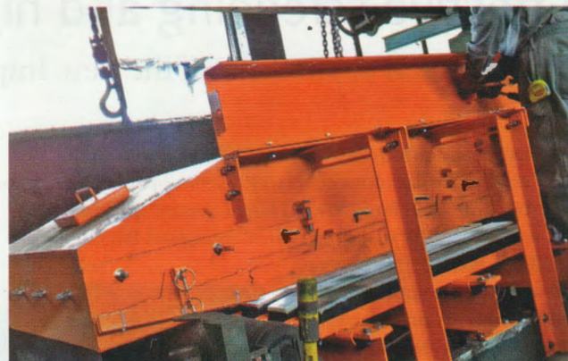
4 The Martin® Transfer Point Kit can be assembled prior to installation or assembled during scheduled downtime
