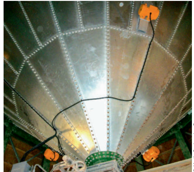
4 Industrial vibrators for bin & chute applications can reduce or even eliminate the need for cleaning
