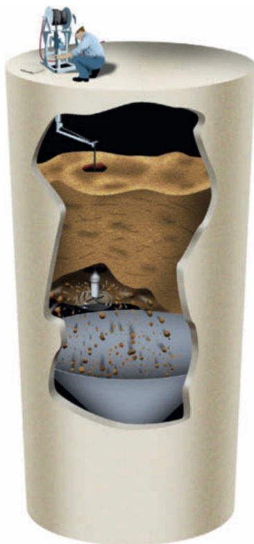
2 Safe, effective cleaning requires tools that work inside the silo from the top, controlled by personnel outside
