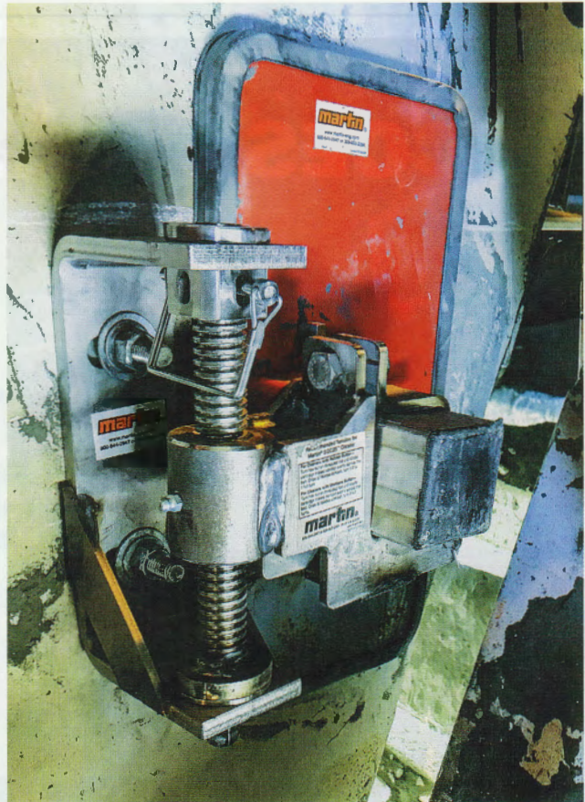
2 The CS2 typically requires just one re-tensioning during its lifespan, helping to reduce cost of ownership
