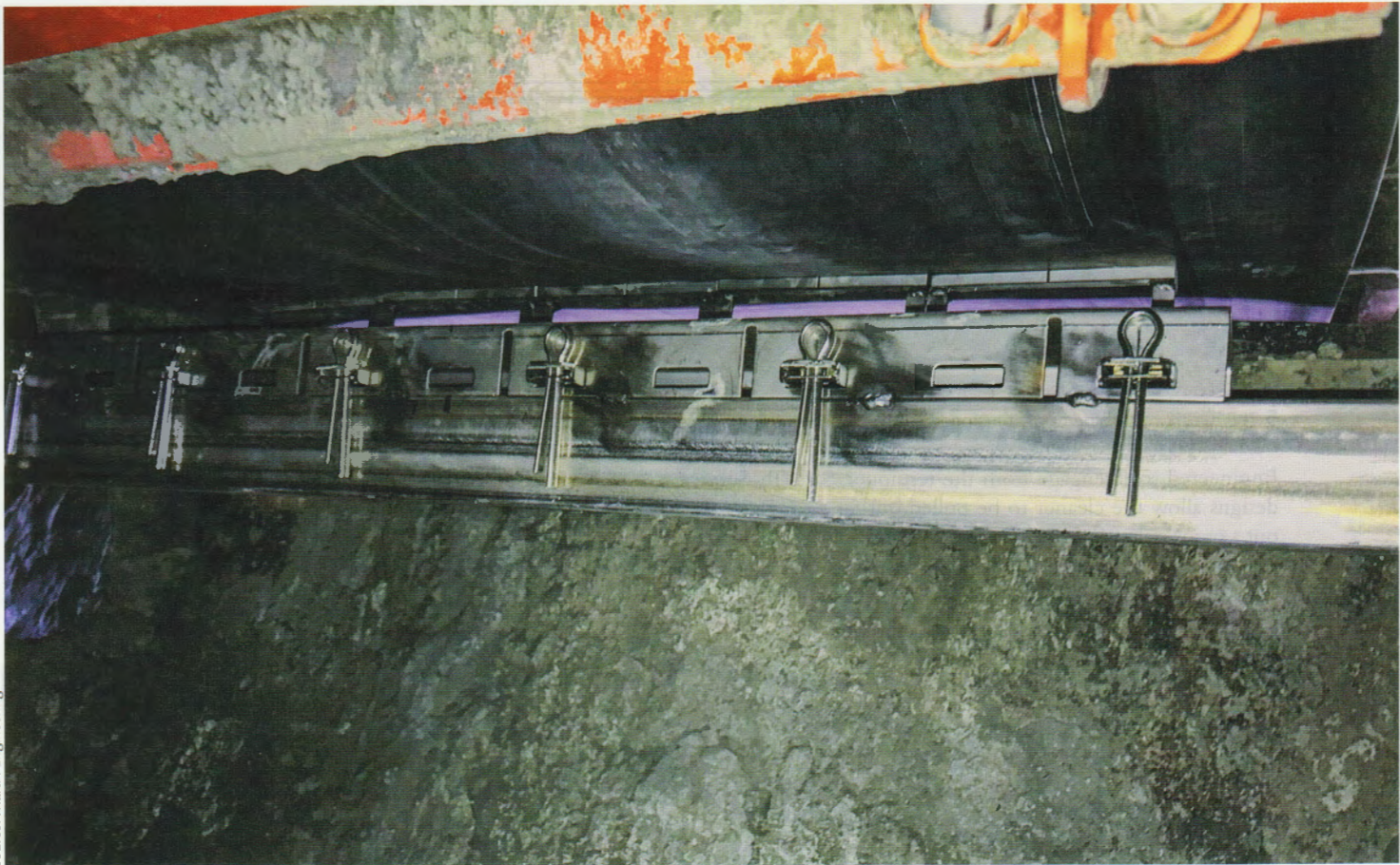
3 The stainless steel design incorporates a matrix of spring-loaded carbide tips
