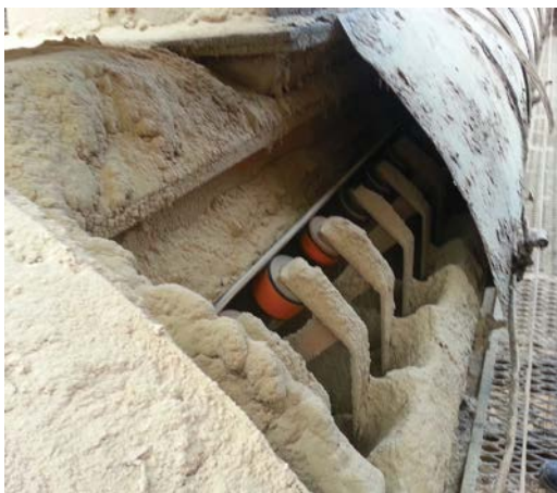
Dust and spillage clog idlers, requiring them to be replaced and raising the cost of operation.
