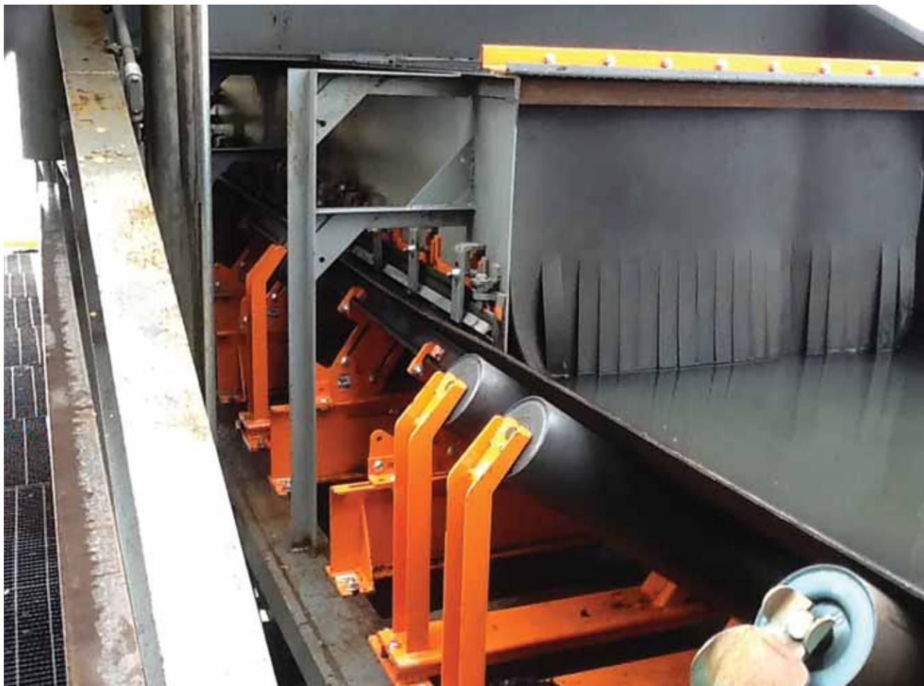
concussion of material on the belt, most high-volume operations need one or more impact cradles to absorb the force of the cargo stream. Heavy duty impact cradles
