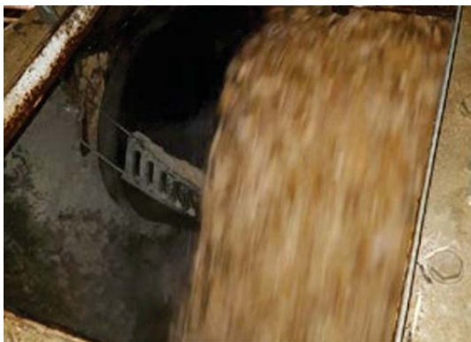
By removing fine material from the belt, more product is captured in the discharge flow.
