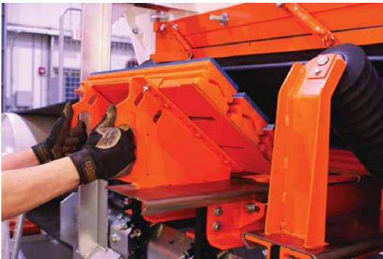
The modular impact cradle absorbs the impact of the falling load, yet slides in and out for easy service.
