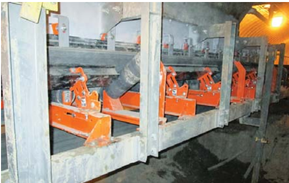
The external skirting system contains fine particles and creates a more stable stilling zone.
