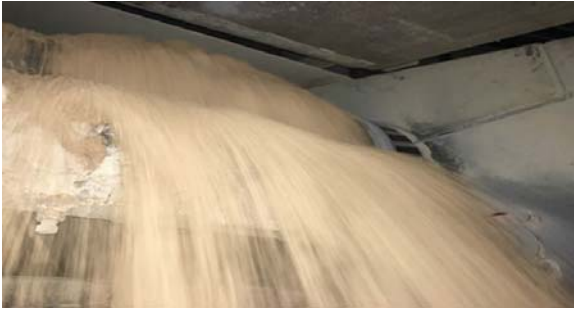
The JEA plant was having chute clogging and spillage issues at the discharge zone of its limestone conveyor.
