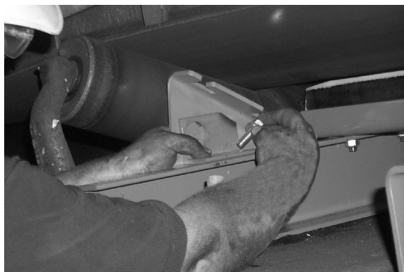
14. Bolt on the fine tune adjustment angle but do not tighten.
