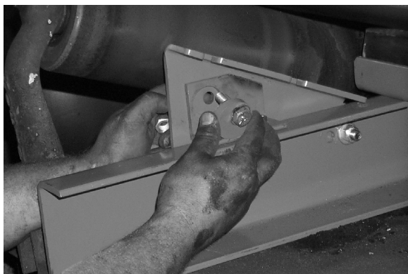
14. Bolt on the fine tune adjustment angle but do not tighten.
