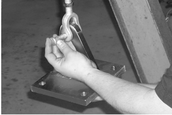
11. Assemble top mount weldment to turnbuckle.
