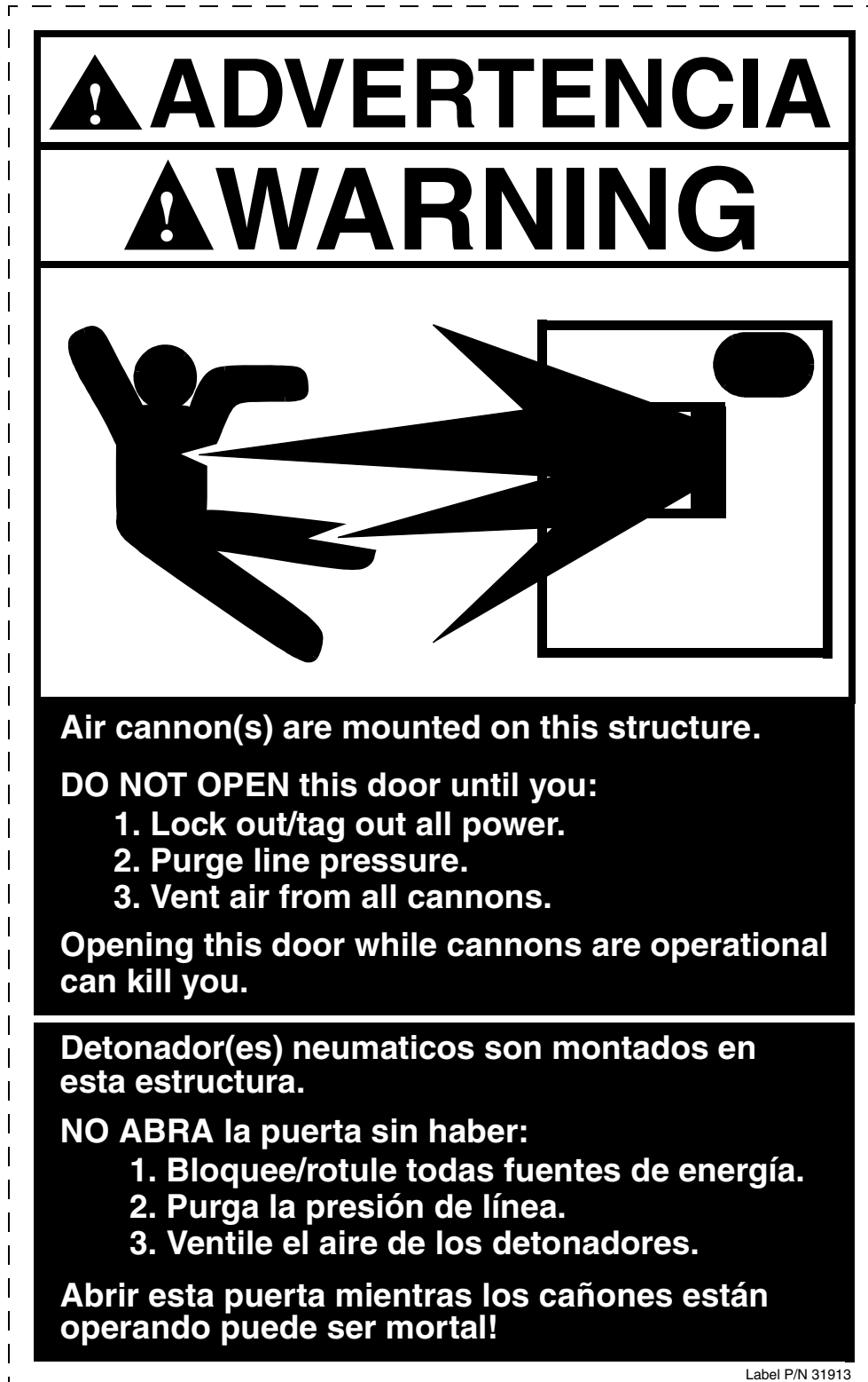
Figure 22. Air Blast Warning Label, P/N 31913
