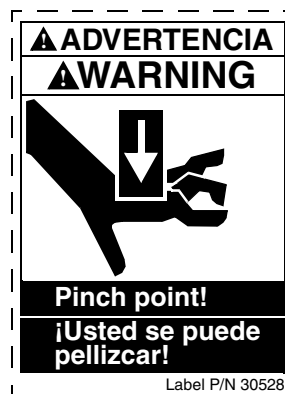
Figure 3. Pinch Point Warning Label, P/N 30528
