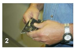
2. Pull the Pin and Knead Components Together All it takes is three minutes.
