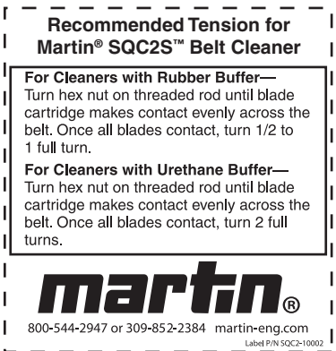
Figure 9. Martin® SQC2S™ Tensioning Label, P/N SQC2-10002
