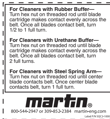
Figure 7. Martin ® SQC2S ™ Tensioning Label, P/N SQC2-10002
