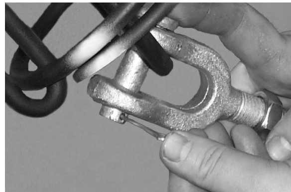
10. Assemble turnbuckle to spring.
