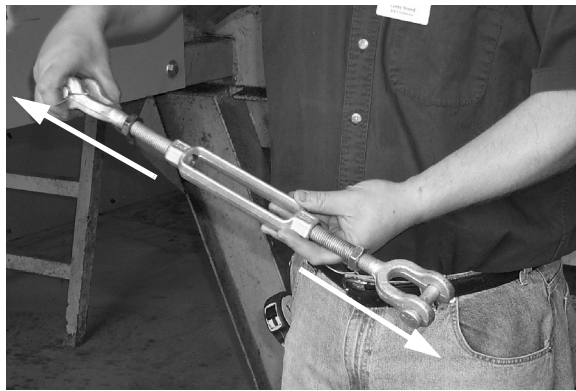
9. Fully extend turnbuckle.
