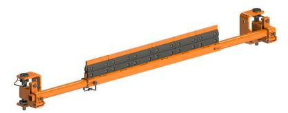
The Martin® SQC2S™ Reduced Mini Cleaner incorporates individually-cushioned tungsten carbide blades for effective cleaning without risk to belt, splice, or blade. Installed in the secondary cleaner position, the Martin® SQC2S™ Cleaner's blade buffers cushion impact and maintains cleaning pressure.
