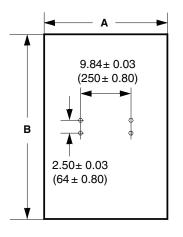
Dribble Sheet Liner available in UHMW polyethylene or high-density polyethylene. Also available with or without drilled holes.
