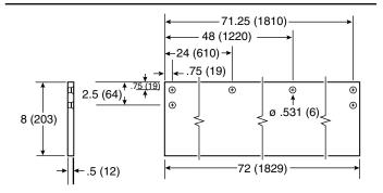
UHMW Polyethylene Wear Liner (standard mounting holes) P/N 32054-XX
