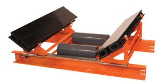
The Martin<sup>®</sup> Modular Slider Cradle utilizes low friction UMHW bars to support the belt at the outside of the loadcarrying area. This stabilizes the belt line, eliminating the sag and bounce that spill material, and reducing the risk of catching lumps that can abrade the belt surface.
