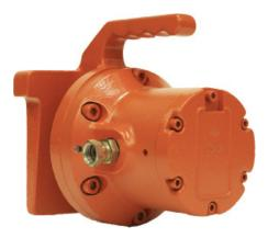
The Martin<sup>®</sup> Impacting Railcar Vibrator delivers a powerful force output of 3400 lbs at 80 psi while only weighing 48 lbs, making it the highest-force, lowest-weight portable railcar vibrator available. The Martin<sup>®</sup> Impacting Railcar Vibrator provides the force required to activate the free flow of tough materials that are sticky, coarse, and high in moisture.
