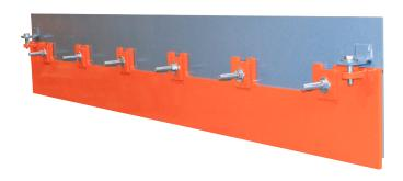
Installed outside conveyor transfer point skirtboards, Martin®\_External Wear Liner Retrofit Kit is an economical upgrade that improves skirtboard sealing and prevents spillage. Wearliner can typically be installed without requiring work inside chute or interfering with existing chute supports.
