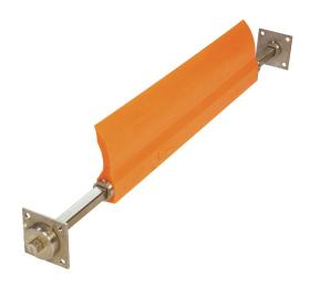
The <u>Martin</u><sup>®</sup> <u>Compact Cleaner</u> from Martin Engineering uses a low-profile blade mounted on an internal square mainframe for effective belt cleaning in tight spaces. It is designed for applications on small pulleys and belts operating at speeds up to 350 fpm (1.78 m/sec).
