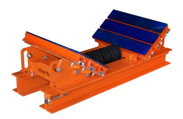
Installed under a belt conveyor loading zone, the <a href="Marting">Marting</a> Combination Cradles absorb the force of falling material to prevent damage to the belt and structure. The impact cradles stabilize the belt line to prevent material escape.
