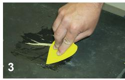
3. Apply to Surface Cut corner and spread with brush, mixing stick, or tool. Pot life is approximately 10 minutes.
