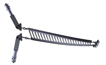
The <u>CleanScrape<sup>®</sup> Cleaner</u> is mounted diagonally on the discharge pulley and forms a three-dimensional curve. The cleaner has a matrix of carbide scrapers incorporated into the main rubber body during the vulcanization process. Despite a relatively low contact pressure between the belt and cleaner 85 to 95% of the adhering material is removed.
