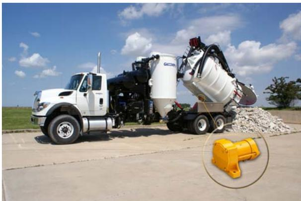
*Although Vactor uses four different vibrator models for various applications in its vacuum loaders and hydro excavators, all are Cougar® vibrators. Each industrial truck gets a mounting plate, whether ordered with a vibrator or not, so a retrofit is an easy bolt-on installation*
