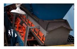
With its slide-in/slide-out cradles and external wear liner, the EVO® Conveyor Architecture simplifies maintenance.
