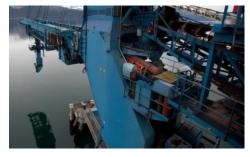
To improve flow and reduce the escape of dust and spillage, Aurora Energy Services authorized improvements to the shiploader's boom conveyor.
