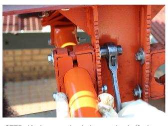
STEP 12: Loosen the bolts on the half clamp that were tightened earlier in order to secure the scraper.
