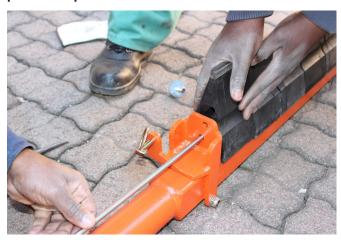
STEP 6: As recommended by CEMA the secondary scraper is most effective when positioned as close as possible to where the belt exits the head pulley. If possible within 50mm of this would be the ideal position. If the scrapers are to be installed on a closed chute application then you would need to make a cut out of minimum 150mm x 300mm, if using a double scraper remember to measure the distance of both pipes and the distance of the bracket being used.
