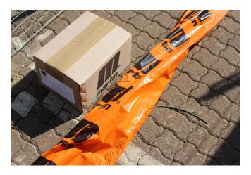
STEP 2: The scraper should be removed from packaging and moved to a level surface (concrete slab, conveyor platform or walkway) where assembly can be performed safely. Clamp both ends of the pipe to prevent the pipe rolling during assembly.
