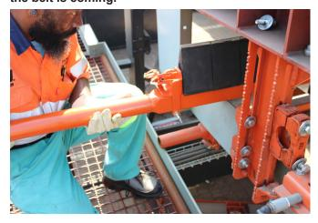
STEP 9: Raise the scraper to the belt so that all blades are just touching the belt. The blades must be at 90 degrees to the belt.
