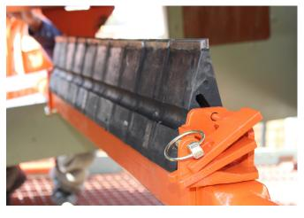
STEP 11: Install the adjusting block onto the bracket. Ensure that the adjusting bolt is flush with the surface that will mate with the clamp. Fasten the adjusting block.
