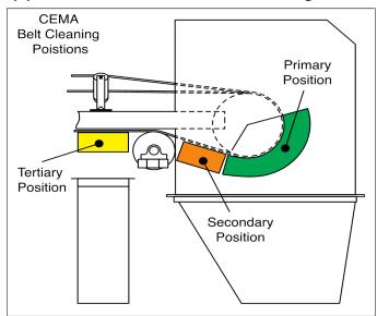
On an open chute application position the bracket as illustrated on the structure. The first scraper should be within 50mm of where the belt exits the head pulley. Attached the support pipe on the bracket and tighten the half clamp bolts. When using the support pipe it is necessary to cut the pipe in order for it to be in the correct position on the belt
