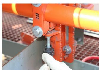
The adjusting bolt must now be turned 2 to 3 turns to raise the scraper and to achieve the correct tension to the belt.
