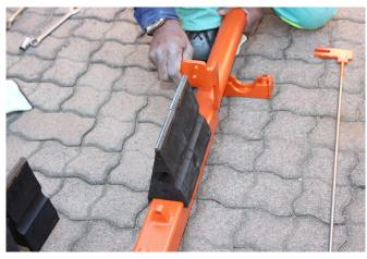
STEP 5: Place the rubber buffer/ blade combination onto the slotted section of pipe and insert the latching pin that is provided to secure them.
