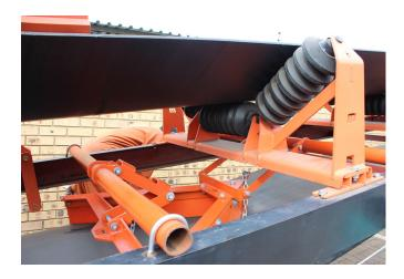
STEP 5: The safety chain must be secured to the pipe. Measure and secure so that when the plough blade is worn there is no possibility of the metal parts of the plough making contact with the belt. Ensure that all the bolts and nuts on the entire plough are fastened. If possible run belt and test the effectiveness of the plough. Make adjustments as required.
