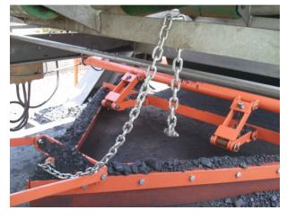
STEP 3: Once the suitable position is chosen place the V Plough onto the belt. Ensure that it does not interfere with other components on the belt and that it will be able to move freely during operation. Place the arms onto the structure and mark the holes needed for the clamp to secure the plough. The holes must be equidistant from each other in order to ensure that the plough rides correctly. The front and rear pipe must be parallel to each other.
