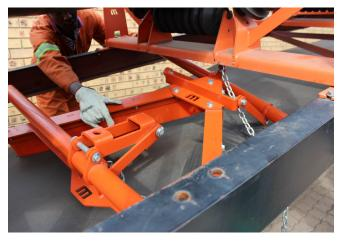
STEP 4: Fasten the clamps and ensure that the plough is able to freely move in order to ride the belt.
