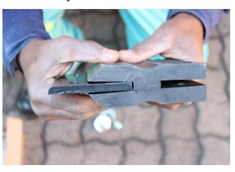
STEP 5: Starting with the middle buffer push the outer buffers toward the outer edges of the pipe. Tighten the centre buffer and then move the outer buffers toward the centre. The blades should not touch each other and should be 0,5mm apart from each other. Tighten the buffers until all have been fastened.
