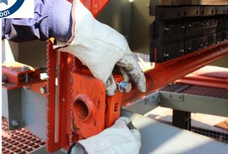
STEP 14: Raise the scraper to the belt so that all blades are just touching the belt. The blades must be at 90 degrees to the belt. Fasten one of the half clamp bolts on either side to hold the scraper in place.
