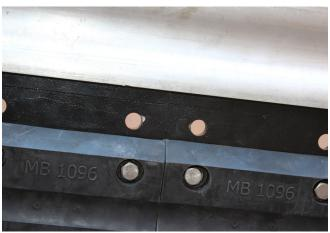
STEP 8: As recommended by CEMA the secondary scraper is most effective when positioned as close as possible to where the belt exits the head pulley. If possible within 50mm of this would be the ideal position. If the scrapers are to be installed on a closed chute application then you would need to make a cut out of minimum 150mm x 300mm, if using a double scraper remember to measure the distance of both pipes and the distance of the bracket being used.
