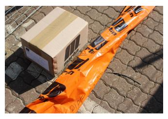
STEP 2: The scraper should be removed from packaging and moved to a level surface (concrete slab, conveyor platform or walkway) where assembly can be performed safely. Install the clamps on both ends of the pipe to prevent the pipe rolling during assembly.
