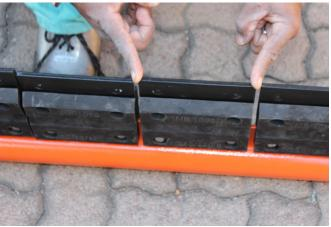
STEP 6: Start with the two outermost blades and lift them up as far as is possible. Finger tighten the bolts and nuts. Place the straight edge on the two outermost blades and by gently bumping the straight edge line and level them. When level, tighten the bolts and nuts.
