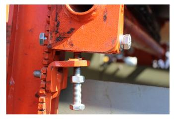
STEP 18: To check for correct tension push one of the blades in direction of belt travel, when released the blade should return and should have a negative angle of attack relevant to the belt. The deflection should not exceed 5 degrees. If it does the belt cleaner is over tensioned
