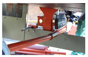
STEP 11: Measure the middle of the scraper and mark it, now measure the middle of the belt and mark it. The difference between the two must now be removed from the support side of the pipe.
