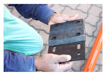
STEP 4: Place the rubber buffers onto the slotted section of pipe and insert the bolts and nuts that are provided to secure them. Do not tighten at this stage.
