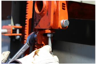
STEP 15: Install the adjusting block onto the bracket. Ensure that the adjusting bolt is flush with the surface that will mate with the clamp. Fasten the adjusting block.
