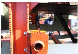
STEP 16: Loosen the bolts on the half clamp that were tightened earlier in order to secure the scraper.
