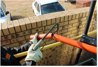
STEP 12: The scraper is now inserted over the support pipe and ready for installation. Ensure that the tungsten on the blade is facing towal head pulley. The direction from which the belowing (indicated with an arrow in image below).
