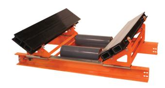
The Martin® Modular Slider Cradle utilizes low friction UMHW bars to support the belt at the outside of the loadcarrying area. This stabilizes the belt line, eliminating the sag and bounce that spill material, and reducing the risk of catching lumps that can abrade the belt surface.
