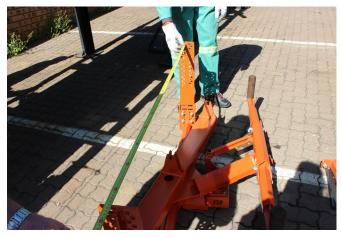
STEP 8: When adjusting the hanging arms loosen the four bolts as indicated above and the move the arms accordingly. Ensure that the correct measurements are met and tighten the bolts.
