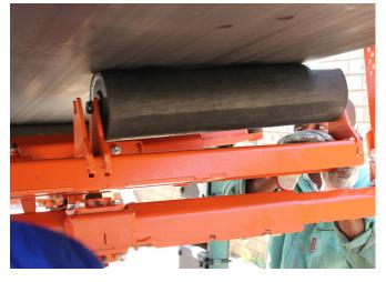
STEP 16: Ensure that the tracker is at the correct height and is free from all obstructions. Tighten all the bolts and nuts.
