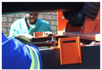
STEP 7: Measure the distance from the outside of the stringers, this measurement can be used to measure how far apart the hanging arms need to be. When making this adjustment remember to make the distance from the middle of the tracker equidistant to the hanging arms. The tracker must be in the middle of the stringers and not the belt.
