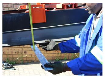
STEP 10: Remember to measure from the top of the idler to the position on the hanging arm.
