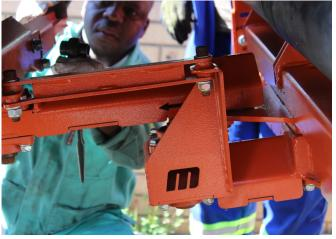
STEP 12: After lowering the steering arms, to make installation easier, maneuver the tracker into position under the belt.
