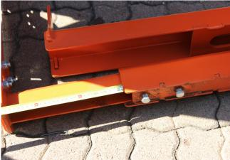
STEP 9: Measure from the top of the stringer to the bottom of the belt. This measurement is how long the hanging bracket should be set to. When adjusting the hanging bracket subtract 10 – 25mm from the total to have the correct setting and to ensure a positive contact between the belt and idlers.
