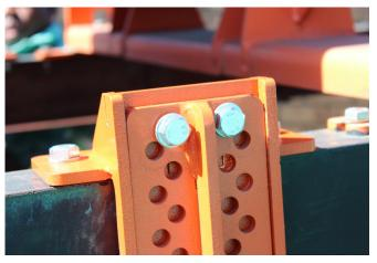
STEP 15: Raise the steering arms to the correct position and tighten the bolts and nuts. Both wing rollers should be 10mm from the belt edge.
