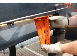
**STEP 4:** Ensure brackets is facing the correct way (arrow to point in the direction of the return belt).
