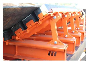
STEP 12: The belt should not ride on the centre bars of the impact bed. It is essential that a gap of between 12 - 25 mm exist between the belt and impact bars when the belt is empty.
