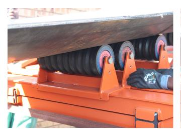
STEP 11: Secure all the idler retainers to the frame as illustrated and tighten all the bolts. Ensure to tighten retainers on both sides of the frame.
