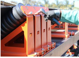
STEP 16: The centre rollers must be in contact with the empty belt, the wing rollers should have a gap of approximately 10 – 13mm between the idler and belt.
