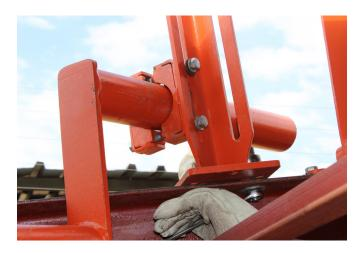
STEP 6: If possible run belt and test the effectiveness of the plough. Make adjustments as required.
