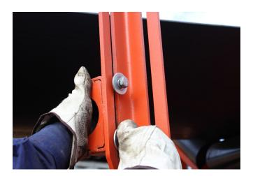
STEP 5: Ensure that all the bolts and nuts on the entire plough are fastened.
