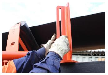
STEP 4: Fasten the half clamp to the bracket and then attach the plough.
