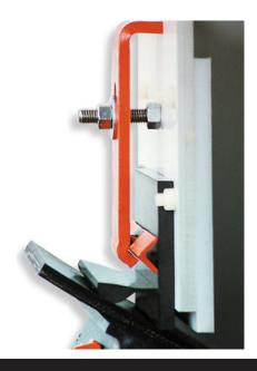
Martin® ApronSeal™ Single Skirting is a dual sealing system that prevents spillage without requiring service to maintain an effective seal. Martin® ApronSeal™ Skirting Systems provide dual-sealing surfaces. The primary seal is clamped to the chute wall with the self-adjusting secondary laying outward to create an effective dust seal that is out of the material flow.
