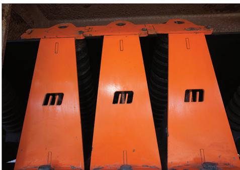
*Innovative patent pending upper connector brackets link idlers together throughout the load zone, allowing them to work together as a unified structure.*
