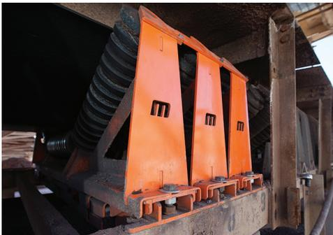
*Elastomer bar suspension allows for defined vertical travel, absorbing shocks from impact maximizing the life of the belt support structure and rolling components.*
