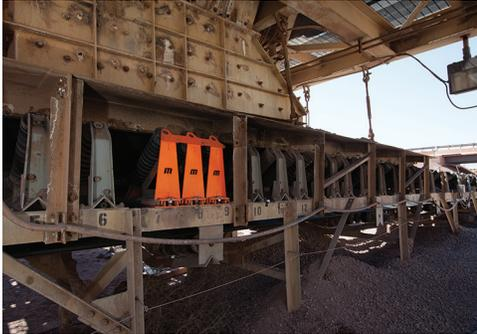
*EVO® High Speed Roller Cradle is designed and engineered for high speed/high tonnage belts.*
