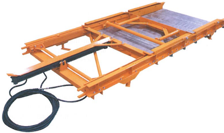
The hydraulic ram of the Carryback Capture System moves a plough across the collection tray to return material to the main cargo stream.
