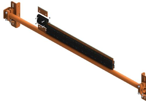
**STEP 5:** Loosen bolts that attach the clamp to the bracket, on the side that does not have the standard support pipe.
