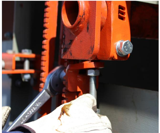
**STEP 30:** Tighten all setscrews and nuts either side of scraper.
