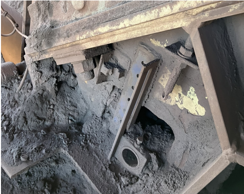
Material spillage demanded frequent manual clean-ups, driving up labor costs and posing serious safety risks.
