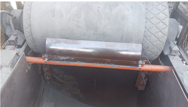
Martin® QC1+™ Cleaner HD with Constant Angle Radial Pressure (CARP) technology
