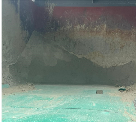
Material stuck in the bin due to its sticky and abrasive nature, causing several operational challenges
