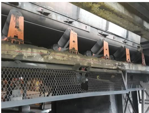
The Trac-Mount™ Idlers are proving effective at containing fugitive material.
