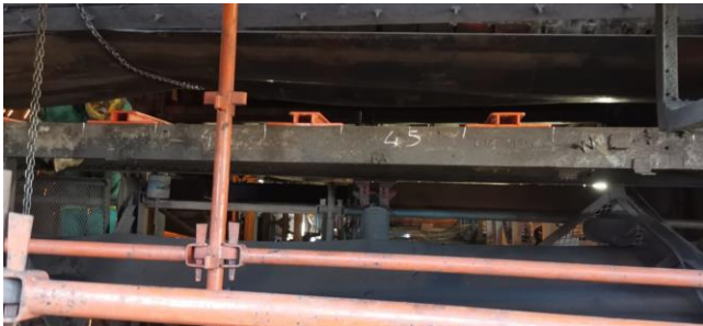
The Trac-Mount™ Idlers strategically placed to ensure proper belt support.
