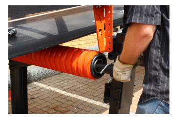
6. Place U-bolt into holes on either side.
