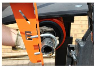
8. Rotate central shaft of Roller Tracker so the machined flats on the shaft are parrallel with indicator on bracket (approximately 30 degrees towards the direction of the return belt).
