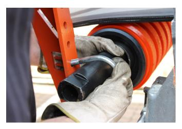
7. Loosly fasten the Roller Tracker using the U-bolts equally on both brakcets.
