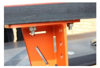
5. Set height of Roller Tracker approximately 5 mm higher than the removed return idler. Ensure Roller Tracker is in the center of the stringer (use stringer as guide and NOT the belt).
